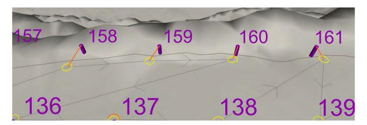
Many mines struggle with drill and blast data. With 50 or more data points per hole and thousands of holes fired each week, the volume of data can build up fast. The most fundamental of this information is the location of the drillhole.
